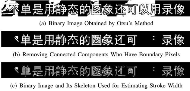
Fig. 2. The method to get binary image and its skeleton used for estimating stroke width.
